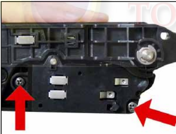
Remove screws holding down the contact plate.
