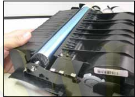
4. With one hand pull the hopper section out while holding the drum section steady then repeat with the second post. Pull hopper straight out to liberate the white bearings inside.
