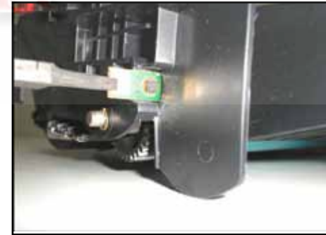
Please remember to replace the chip before installing your cartridge back into your printer.
