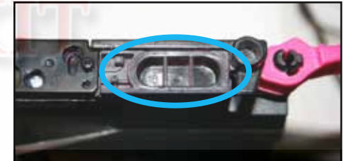
Carefully Remove Plastic Plug
