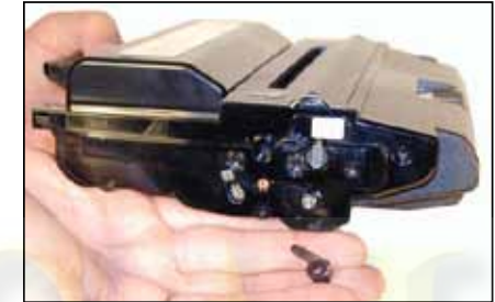
B.. Gently pry off the plastic drum axle bushing. Keep this bushing with the appropriate end cap when removed. Each side is different.
