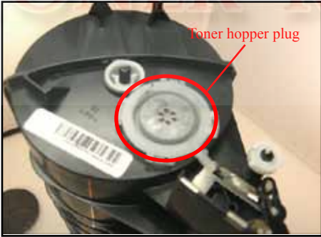
6. Remove the complete white fill plug at the side of the hopper. This is done by prying it open at the base near the border of the hole using a small flat head screwdriver. Opening the breather section (top portion of plug) does not gives access to the hopper.
