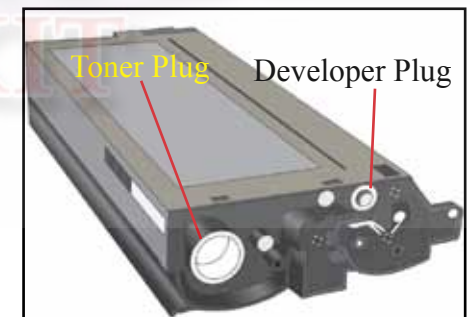
Remove Toner and Developer plugs
